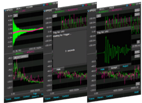
Figure 5: Acquisition Modes 'Free-Run', 'Auto-Trig-ger', and 'Manual Trigger'
